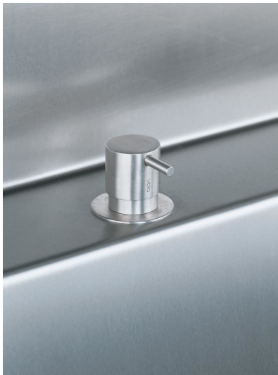
S50 Stop valve with 1/4 turn ceramic disc technology. Includes non-return valve and 1/2" inlet/outlet. 60 mm circular flange 001G. Hole cut out size: 30 mm.
