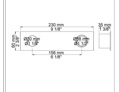
**4002L** Two-hole plate 60 x 231 mm. Holes Ø30 mm and Ø38 mm for 4800.
