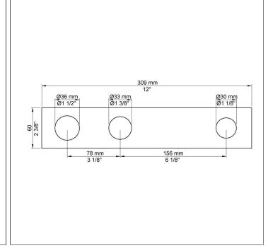
**3003** Three-hole plate, 60 x 309 mm. Holes Ø36, Ø33 and Ø30 mm.
