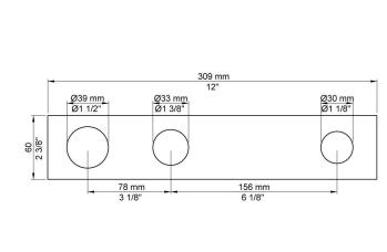
**2003** Three-hole plate, 60 x 309 mm. Holes Ø39, Ø33 and Ø30 mm.
