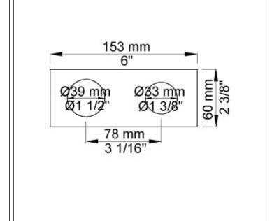
**2002** Two-hole plate, 60 x 153 mm. Holes Ø39 and Ø30 mm.
